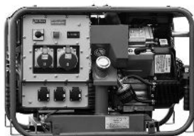
14 kW Mobile Generator - Inverter technology 230/400V with one 3 phase 32 Amp plug, one 3 phase 16 Amp plug and three 16 Amp schuko plugs
